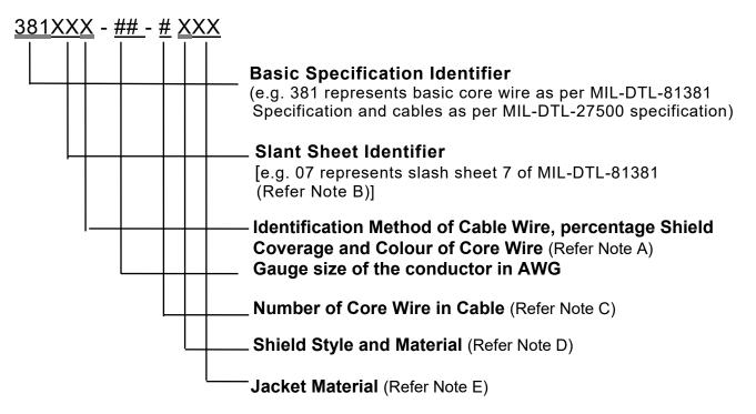
**Example : 38107D-22-3SKK** = 22 AWG, 3 core wire (White, Blue, Orange) as per MIL-DTL-81381/7, Silver plated Copper shielded with 90% coverage, jacket of natural Polyimide tape combined with FEP having Polyimide as a outer surface and heat sealed
